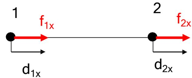
A distributed load is represented by two nodal loads in a consistent manner
