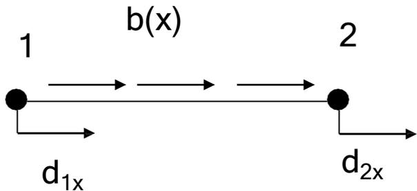
$$\underline{f}_b = \int_{x_1}^{x_2} \underline{\mathbf{N}} \mathbf{b} \, dx = \int_{x_1}^{x_2} \begin{Bmatrix} N_1(x) \\ N_2(x) \end{Bmatrix} \mathbf{b} \, dx$$
