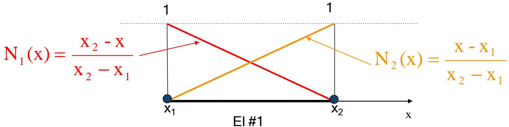
**Within the element, the displacement approximation is**
