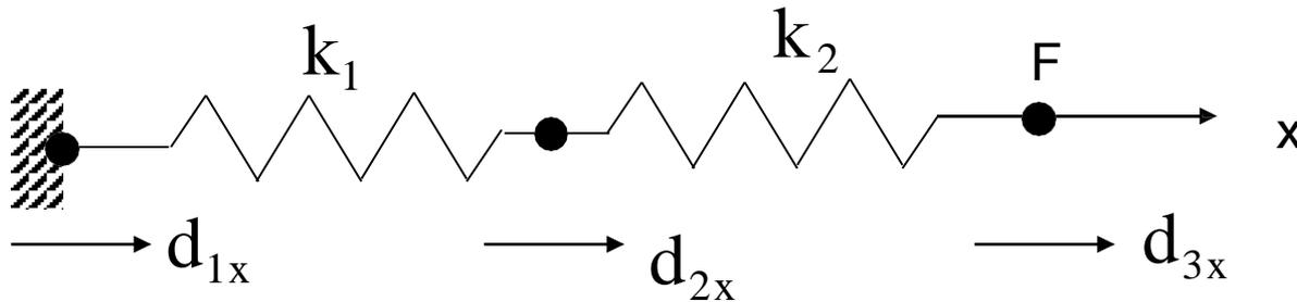
For this system of spring, first write down the total potential energy of the system as:
