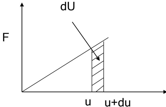
Differential strain energy of the spring for a small change in displacement ( $du$ ) of the spring
