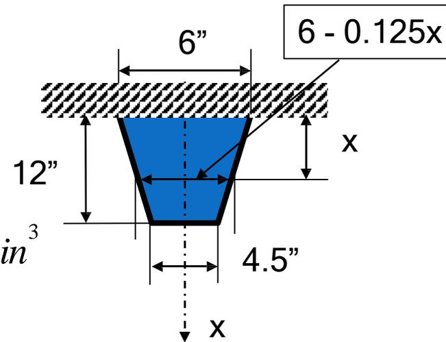
Now compute the element load vector due to distributed body force (weight)
