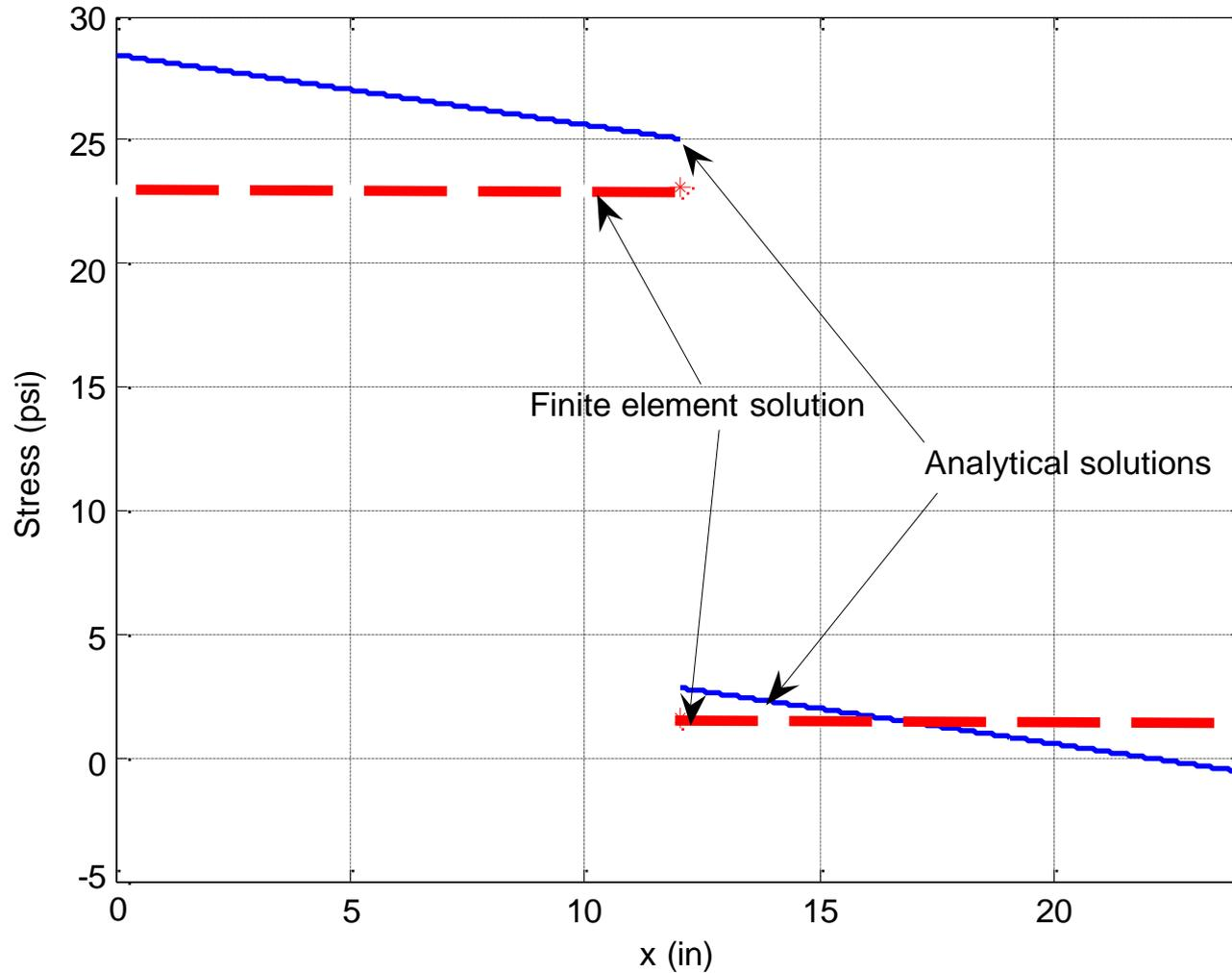
The analytical as well as the finite element stresses are discontinuous across the elements
